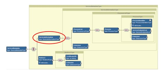
This input structure, from the *ServiceInformation* node down to the Process' leaves will <u>fully</u> define the content of the referenced service metadata as defined by the four identifiers of the participant AND related specific document.
