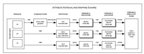
The main tasks of the service include the retrieval of the data from the hardware token (READ), optionally the decompression of stored data (DECOMPRESS), the parsing of information fields (PARSE), the mapping of attributes into a normalized form (MAP) and finally the embedding of those attributes into a predefined container format.
