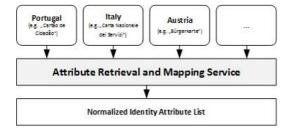
The service is able to map attributes stored in different formats (e.g. subject-DN of X.509 certificate, BCD encoded data or a proprietary XML format) and different places (e.g. proprietary EFs) on to a set of well defined attribute types in a well defined format.
